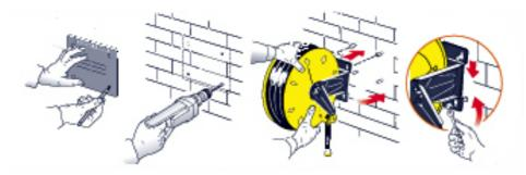
The **solid end compact** fixed bracket, included with the hose reel, is provided with four slotted mounting holes for **easy and safe installation**. Using the template supplied with the hose reel it's easier to mark plugs holes for hose reel
